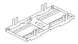
Fold the frames squarely as shown. Reinforce the fold lines with a fillet of solder. Do not fill the slots at the ends of the longitudinals as these are needed for the brake assemblies.
