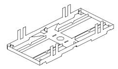
Fold the frames squarely as shown. The frame ends need to be shortened, as marked by the half-etched lines. Reinforce the fold lines with a fillet of solder. Do not fill the slots at the ends of the longitudinals as these are needed for the brake assemblies.
