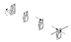
Fold up the bearing carriers as shown. Solder in the waisted bearings, then push the top tabs forward slightly. Thread two carriers onto a length of the supplied spring wire and gently squeeze the tabs with pliers to hold the carriers in place.
