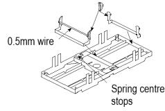
Fold up the brake shoe stretchers as shown. Laminate shoes either side of the stretchers, using the supplied 0.5mm wire cross shafts for alignment. Fix the shoe assemblies to the frames.
