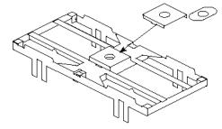
Add the pivot plate and any packing washers as shown.
