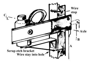
Calling on arms are also pivoted on the left-hand side, but with the lamp on the same side. They may be operated by a pull rod at A as shown, or by a lever B at the rear made from scrap etch.
