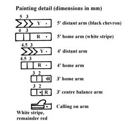
Generally, spectacles and ironwork are black, with posts and dolls white. Rule 55 diamonds had a black band 1' deep above and below. Arm fronts and edges are as shown above. The arm backs are white, with a black stripe or chevron repeating the symbol on the front. Discs are all white with a horizontal red stripe on the front. For both arms and discs, the top lens is glazed red (yellow for distants), and the bottom one green.
