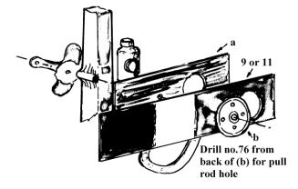
The restricted clearance arms 9 and 11 are mounted with the spectacle frame behind the arm as shown above.
