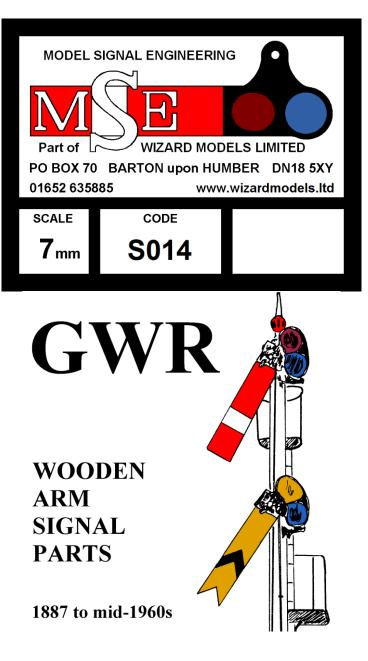
These wooden arms, on wooden posts, were the most common style in the heyday of the Great Western Railway. From the 1930s onwards, they were replaced by the new steel arms, at first on the original posts, and later by steel arms on tubular steel posts. Some are still in use today on the various preserved lines.
