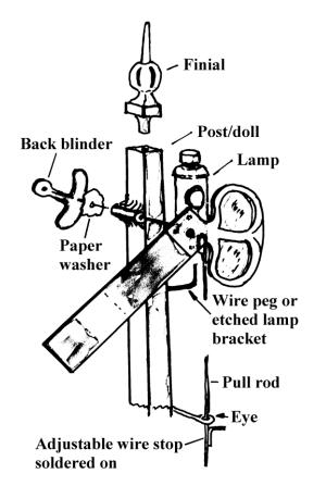
Select the appropriate signal arm, and a spectacle frame. Lay them on the block with a 1.0mm brass wire axle driven through the holes into the wood and solder together. Clear the pull rod hole, using a 5-sided broach for preference. If more than one signal is being made, do a batch, then spray them all over with white matt car undercoat. When dry, the final colours can be applied and the spectacles glazed with MSE *LENS* material. Set aside until the posts are complete.
