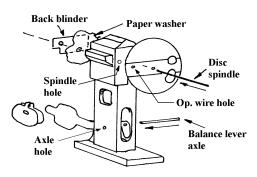
Clean any mould lines or flash from the body casting, and open out the marked holes to no.76 (0.50mm). Open out the holes in the corner of the etched balance lever and the back blinder to no.76 (0.50mm). Tin (145°) the balance weight, fold it in half, and solder (145°) it to the lever as shown, with the holes to the top.
